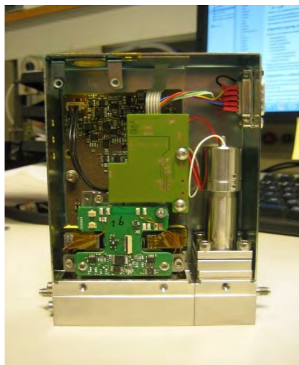
Figure 1. Inside of the flow controller with visible piezo valve
