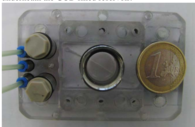
Figure 2: Lab-on-a-chip perfusion system with integrated hollow fiber.
