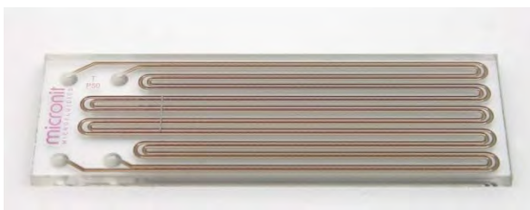
Figure 4: up-scaled EDGE chip containing copper parts as a first step toward fully metal emulsification micro systems
