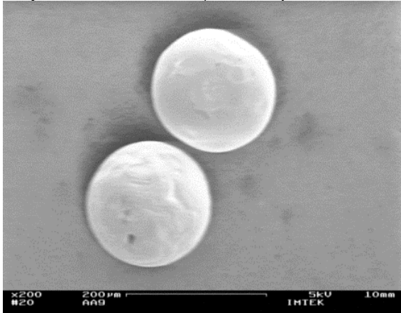
Figure 3: Droplets from Zamak ( d = 180 \mu\text{m} ), printed using the StarJet technology.
