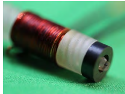
Figure 6: Prototype of the disposable, non-contact dispensing valve fabricated applying a 3D printing process.
